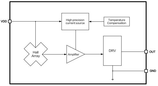
Figure 3. Function Block Diagram of XL47T
