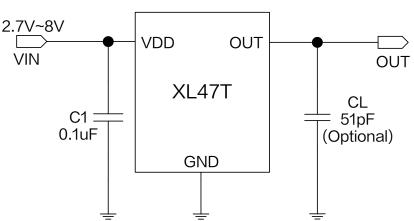
Figure 1. XL47T Typical application schematic
