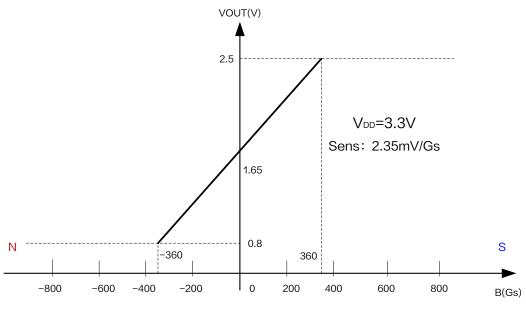
Figure 5. Output Characteristic Curve of XL47T
