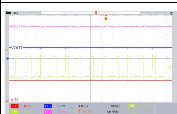
Figure32. LED Current Ripple ( V_{IN}=24V , V_{OUT}=6.6V , I_{OUT}=0.3A )
