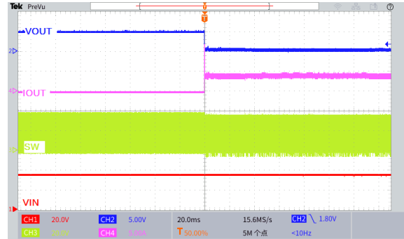
Figure 25. Output Short Circuit Waveform ( V_{IN}=36V , V_{OUT}=5.0V )
