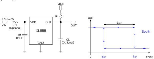
Figure 1. XL558 Typical application schematic and output characteristic curve
