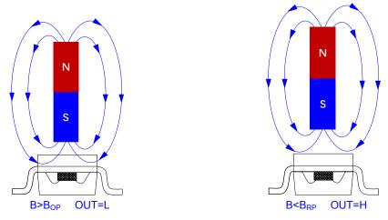
Figure 4. Magnetic Field Direction Definition
