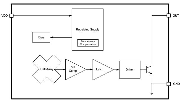
Figure 3. Function Block Diagram of XL558
