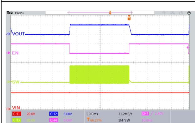
Figure38. Start or Shutdown Using EN Pin
