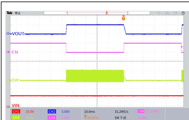
Figure36. Start or Shutdown Using EN Pin
