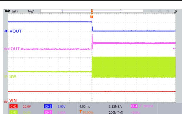
Figure29. Output Short Circuit Waveform
