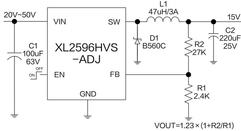
Figure6. XL2596HVS-ADJ System Parameters Test Circuit( $V_{OUT}=15V$ )
