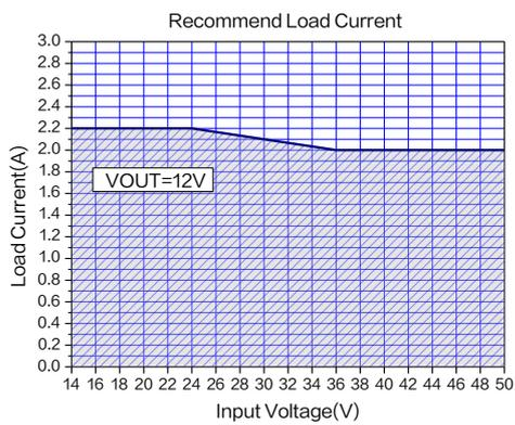
Figure 22. Max Output Current
