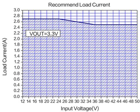
Figure 20. Max Output Current
