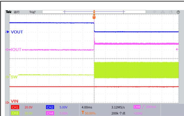
Figure30. Output Short Circuit Waveform
