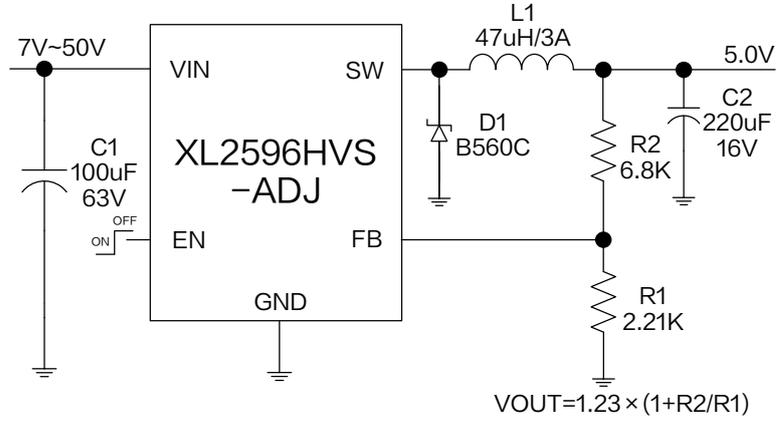
Figure4. XL2596HVS-ADJ System Parameters Test Circuit( $V_{OUT}=5.0V$ )
