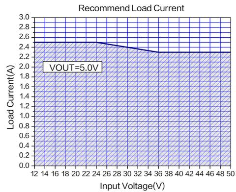
Figure 21. Max Output Current
