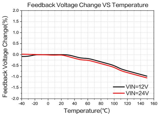
Figure18.Feedback Voltage Regulation
