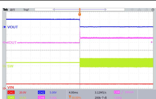
Figure28. Output Short Circuit Waveform
