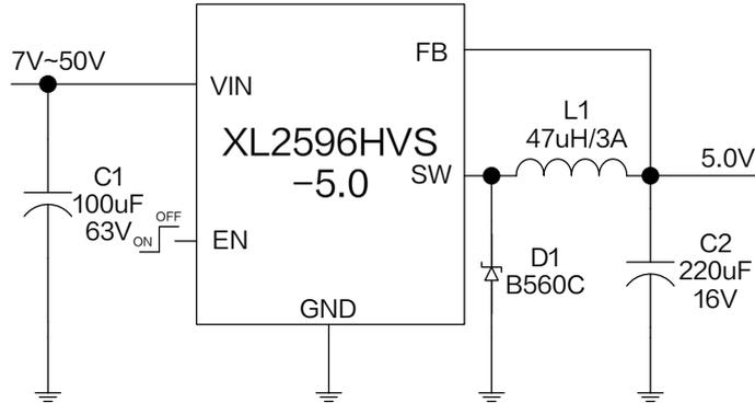
Figure10. XL2596HVS-5.0 System Parameters Test Circuit
