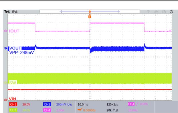
Figure33. Load Transient Response
