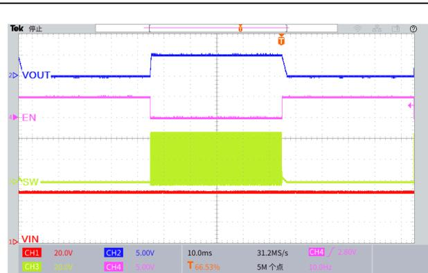
Figure39. Start or Shutdown Using EN Pin
