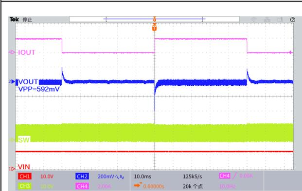
Figure32. Load Transient Response
