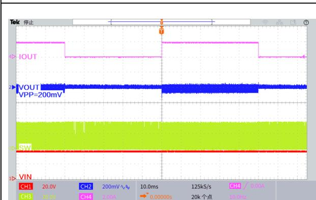
Figure34. Load Transient Response
