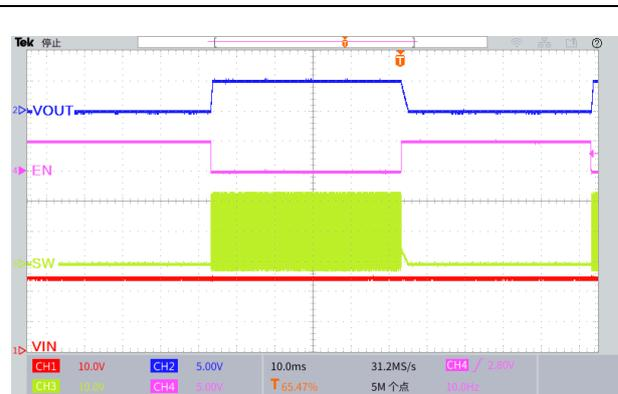
Figure37. Start or Shutdown Using EN Pin
