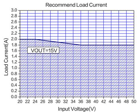
Figure 23. Max Output Current
