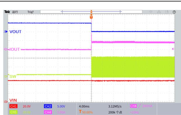
Figure31. Output Short Circuit Waveform
