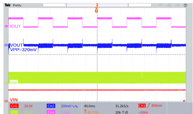
Figure27. Load Transient Response ( V_{IN}=24V , V_{OUT}=5.0V , I_{OUT}=0.1 to 1A )
