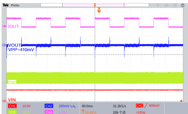
Figure26. Load Transient Response ( V_{IN}=12V , V_{OUT}=5.0V , I_{OUT}=0.1 to 1A )
